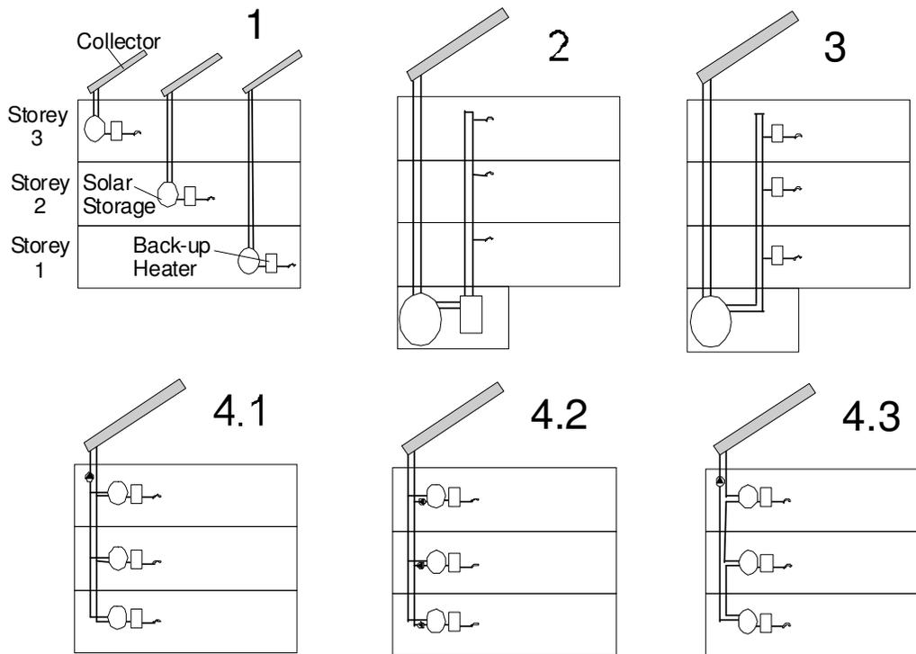
**Figure 3:** Overview of analysed system configurations for MFH
